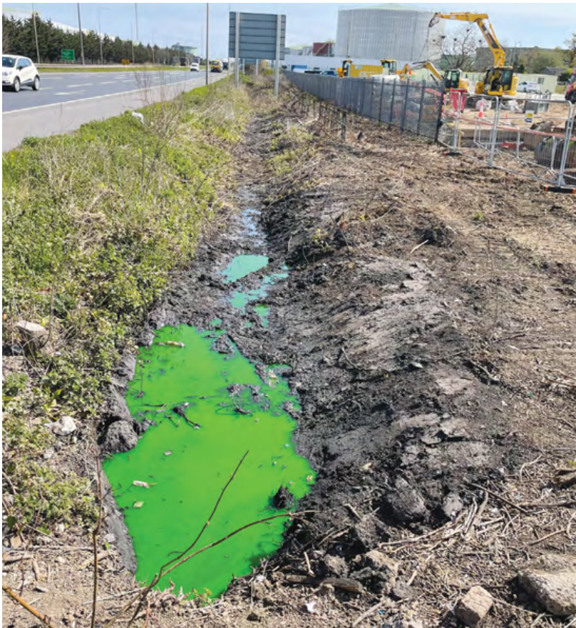
Dye-testing confirmed the interceptor had been incorrectly draining to a drainage ditch on the northern boundary
